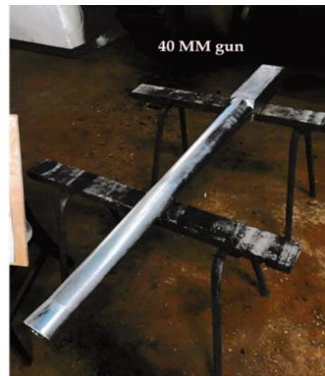
The restoration would involve making a replica of the top half of E1 which included fabricating the driver's compartment, the turret ring support and the engine deck. Also, the complete turret had to be fabricated together with the mantlet and 40mm gun. Although it would be built out of fibre glass and heavy ply and lots of bolts, the finish needed to look like a very rough casting, as these were the first large tank castings ever to be made in Australia.
