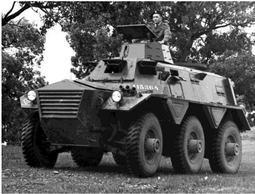
**A Saracen Armoured Personnel Carrier showing the one man turret with the aperture for mounting the machine gun. Smoke grenade dischargers are mounted on the mudguards.**
