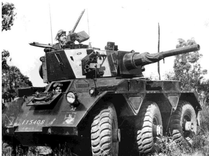
**A Saladin Armoured Car with turret traversed and showing the four wheeled steering. The vehicle mounts a .30inch machine gun operated by the crew commander, and the smoke grenade dischargers can be seen on the turret.**
