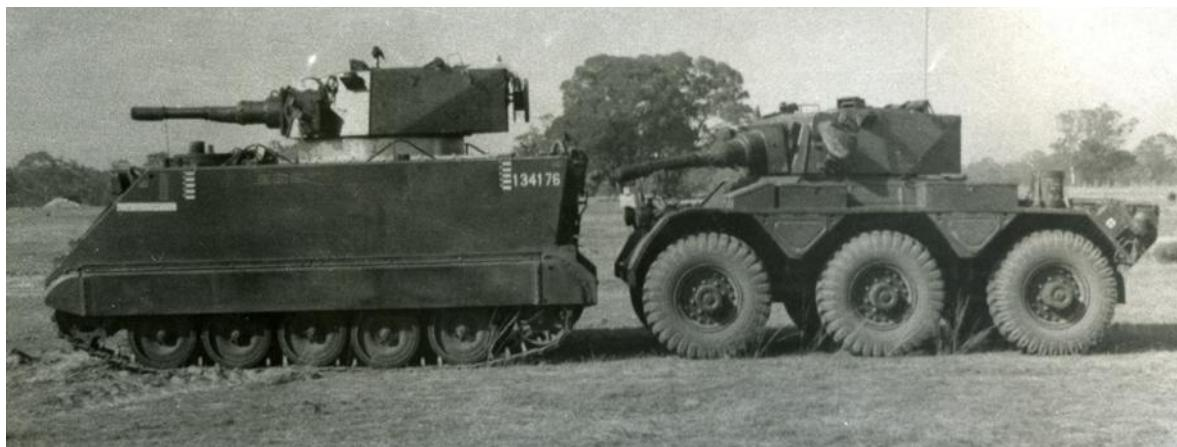
**A Saladin Armoured car and the first M113A1 Fire Support Vehicle (FSV) showing the difference in height of the two vehicles**
