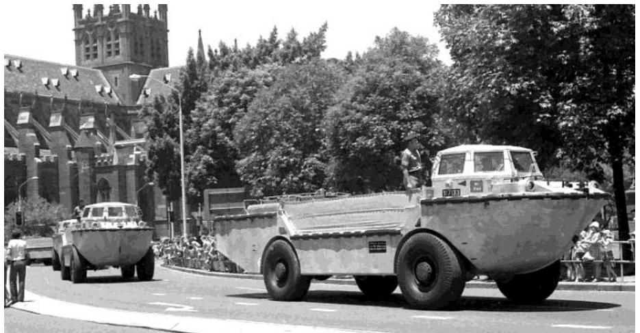
Four LARC Vs of 10 Terminal Regiment during the Queen's Jubilee Parade in Sydney 1977. The original bare aluminium finish of the hull is clearly seen here. (L.A. Wright photo)
