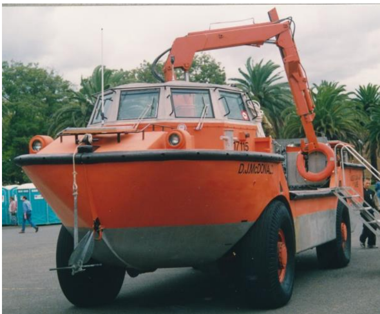
A LARC V of the ANARE Detachment on display at Victoria Barracks, Sydney 1994. This vehicle has the later orange hull top, and the HIAB crane is mounted. (P. Handel photo)
